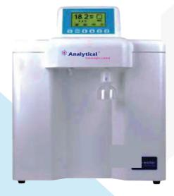
Ultra MS series is popular superior choice of high performance for general analysis pure water. It has 2 kinds of output, 15 or 30 liters/hour. And the resistivity, reaching to 16-18.2M $\Omega$ .cm, is above of the grade I standard of GB6682-2008. It also meets the most requirements of chemical and biological experiments' pure water.
